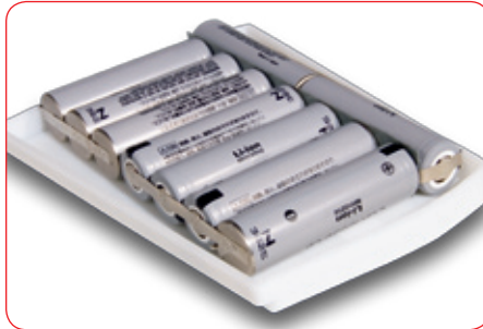
3S3P – lithium-ion cobalt >> 10.8 V and 6,300 mAh
